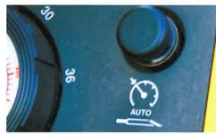
AUTODRILL. Allows the operator to set thrust/ pullback speed, thrust/pullback pressure, or rotation pressure mode while drilling in changing soil conditions. The patent-pending Auto Resume function allows slurry cuttings to mix before thrust/pullback resumes.
