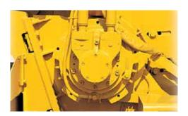
ROTARY POWER TRENCHER DRIVE MOTOR. A rotary power trencher drive motor and splined headshaft produce a lower speed and higher torque which provide superior ground penetration
