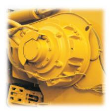
A Rotary Power radial piston hydraulic motor and splined headshaft produce lower speeds and
