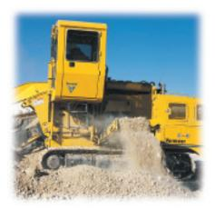
**Nonfolding 8' (2.4 m) or folding 13' (4.0 m) conveyors** offer users maximum flexibility in choosing where the spoil is deposited. The 13' (4.0 m) length gives users the ability to fold the conveyor for easy clearance and storage.
