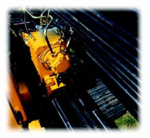
**The D33x44 rack-and-pinion carriage drive** is simple and provides smooth operation. The unique, narrow design of this system helps the unit maintain a small footprint — enhancing access and maneuverability in congested areas.
