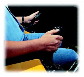
**The operator's station** provides the user with thrust and rotation electronic displacement controls for fingertip operation. Dual-integrated joystick controls combine the breakout system, throttle and mud-flow operations.
