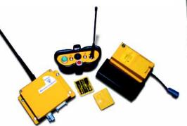
**The Vermeer Remote Lockout System** is a two-way communication and control tool that allows workers to lockout the drill anywhere along the bore path or at the exit site. This patent-pending system is easy to use and is factory-installed in all new NAVIGATOR HDDs; it is available as a kit for installation into HDD machines already in the field.
