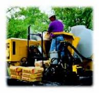
Vermeer drilling fluid systems provide the horizontal directional drill with quality mud mixing in a minimum amount of time. Smaller systems are self-contained on a mounting skid. Larger systems are available preassembled on mounting platforms to provide drilling operations with greater versatility.
